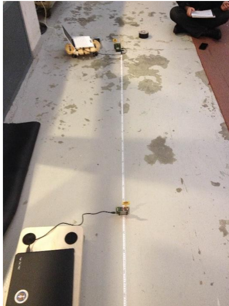
FIGURE 24. The Tape Measure was placed between two Nodes
