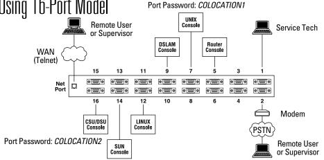
This is just one of many possible installation configurations for the Remote Console Port Manager. In this example, ports have been configured as follows:
