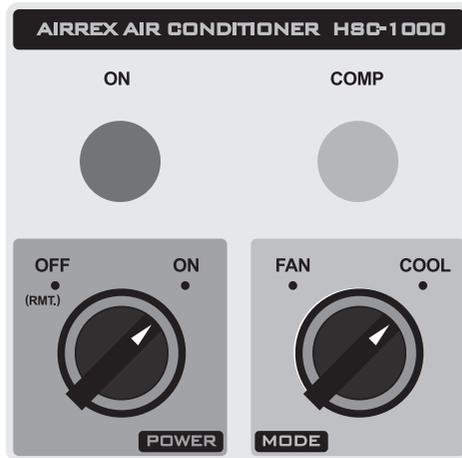
1. ON Lamp : When the air conditioner operates, the Red light is On.
