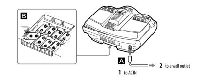
Connect the AC power cord A or insert eight R20 (size D) batteries (not supplied) into the battery compartment B. Notes
