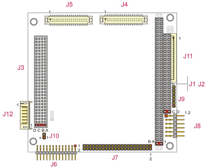
Figure 2. Connector layout
