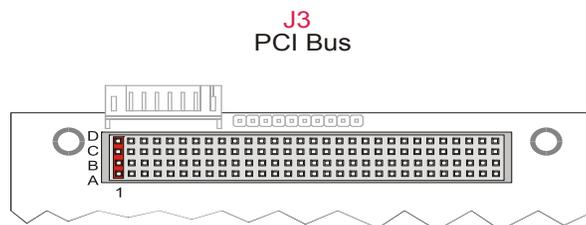
Figure 4. PCI BUS layout
