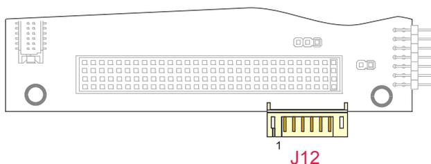
Figure 15. J12 Connector layout
