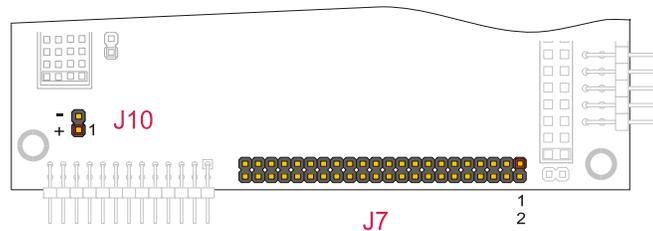
Figure 12. J7and J10 Connector layout
