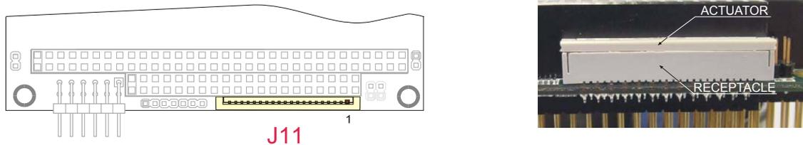
Figure 14. J11 Connector layout
