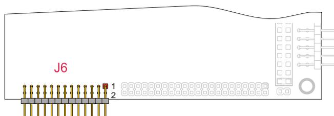
Figure 10. J6 Connector layout
