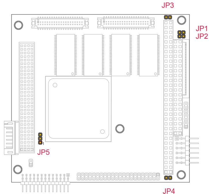
Figure 1. Jumpers and solder jumpers
