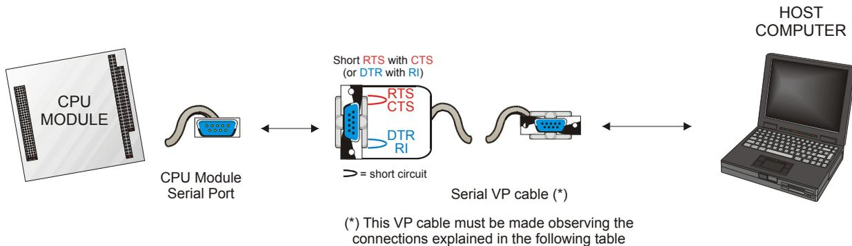
The following table shows the connections required for the cable, we assume that the user is using DB9 cables:
