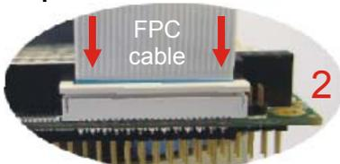
Insert the Flat Printed Circuit cable so that the copper tracks face the PC/104 connector. The FPC connector has contact pins on one side only. The same is true for the connector on the FDD (please refer to the FDD manual for further info). If incorrectly connected, the FDD will not function.
