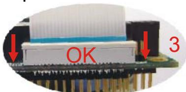
Push down the actuator locking the cable firmly.
