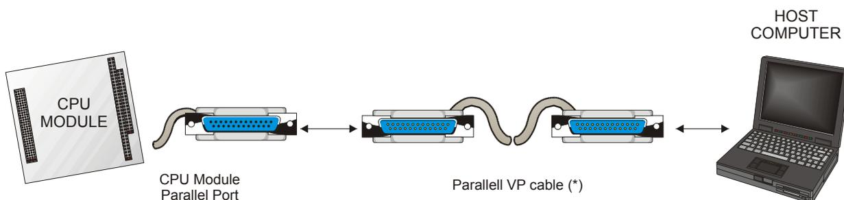
(\* ) This VP cable must be made observing the connections explained in the following table
