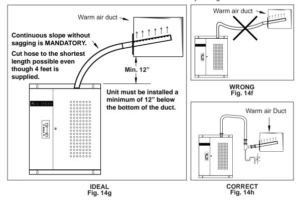
**NOTE**: If it is not possible to get enough slope for the condensation to return properly to the water tank, then an S-shaped steam trap (not supplied) must be installed at the lowest point of the steam hose. This steam trap hose should have a minimum height of 4". Please see <u>Fig. 14h</u>.
