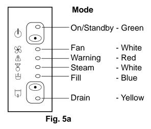
5.2 The ACU-STEAM humidistat also has two pilot lights to indicate the current status.
