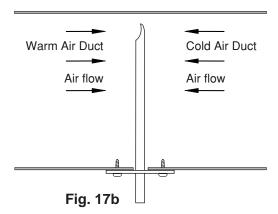
17.5 Push one end of the plastic tube onto the probe outlet. Slip the other end of the tube onto the plastic barbed connector at the end of the tubing already attached to the humidifier for a warm air installation or connect the plastic tube to the LOW barbed connector on the PD Switch located below the electronic control board for a cold air return installation of the probe. Please see <u>Fig. 17c</u>.
