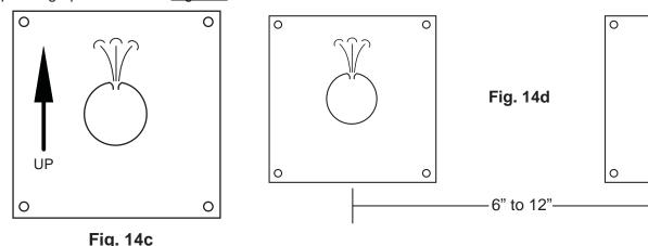
**Note:** Acu-15 models are supplied with two diffusers, hoses and clamps, if there are dual ducts install one diffuser in each duct with equal lenth of hose on each. When installing in the same duct keep a distance of 6" to 12" between diffusers. Please see Fig. 14d.
