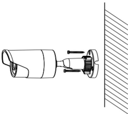
Figure 2-2 Secure the Camera to the Wall/Ceiling
