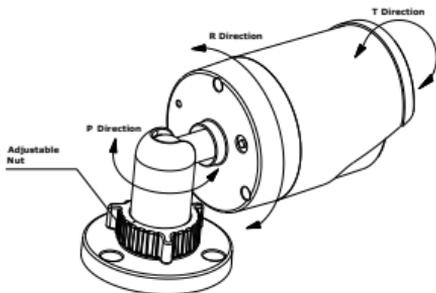
Figure 2-3 3-axis Adjustment
