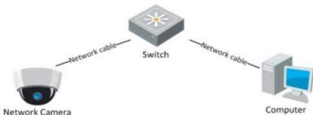
Figure 3-1 Typical LAN Connection
