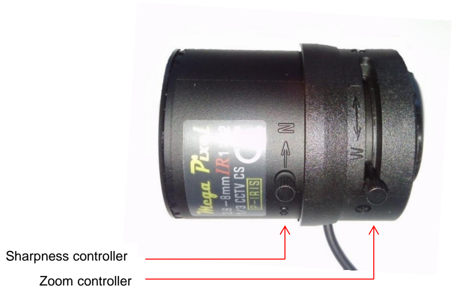
Figure 4.9 Mechanical adjustments at the lens
