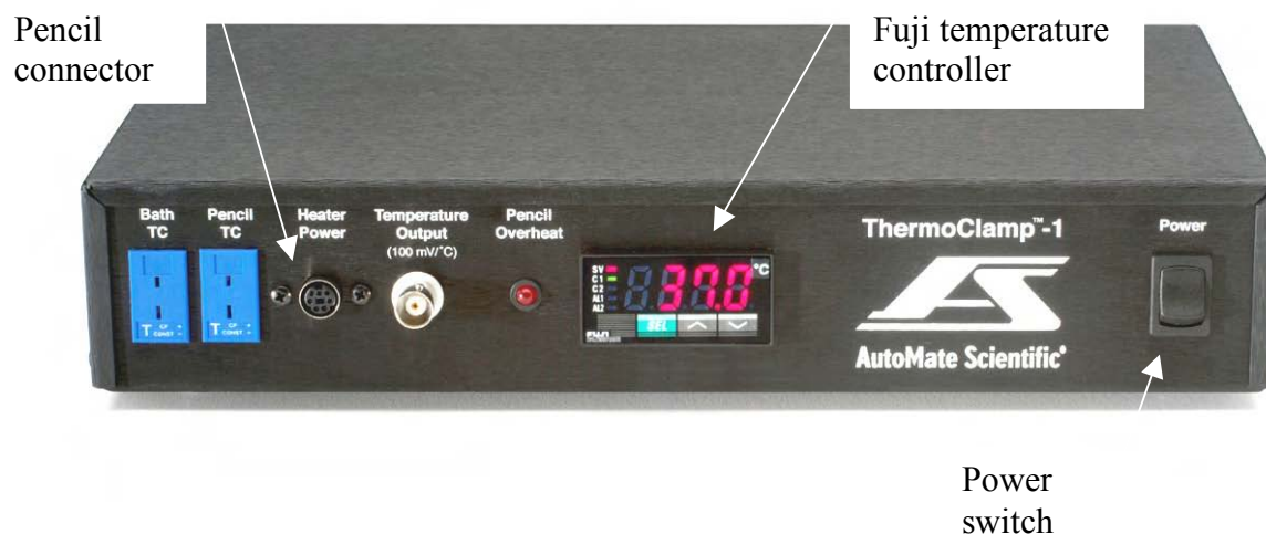
Figure 1. Controller unit, front view. (TC = thermocouple temperature sensor)
