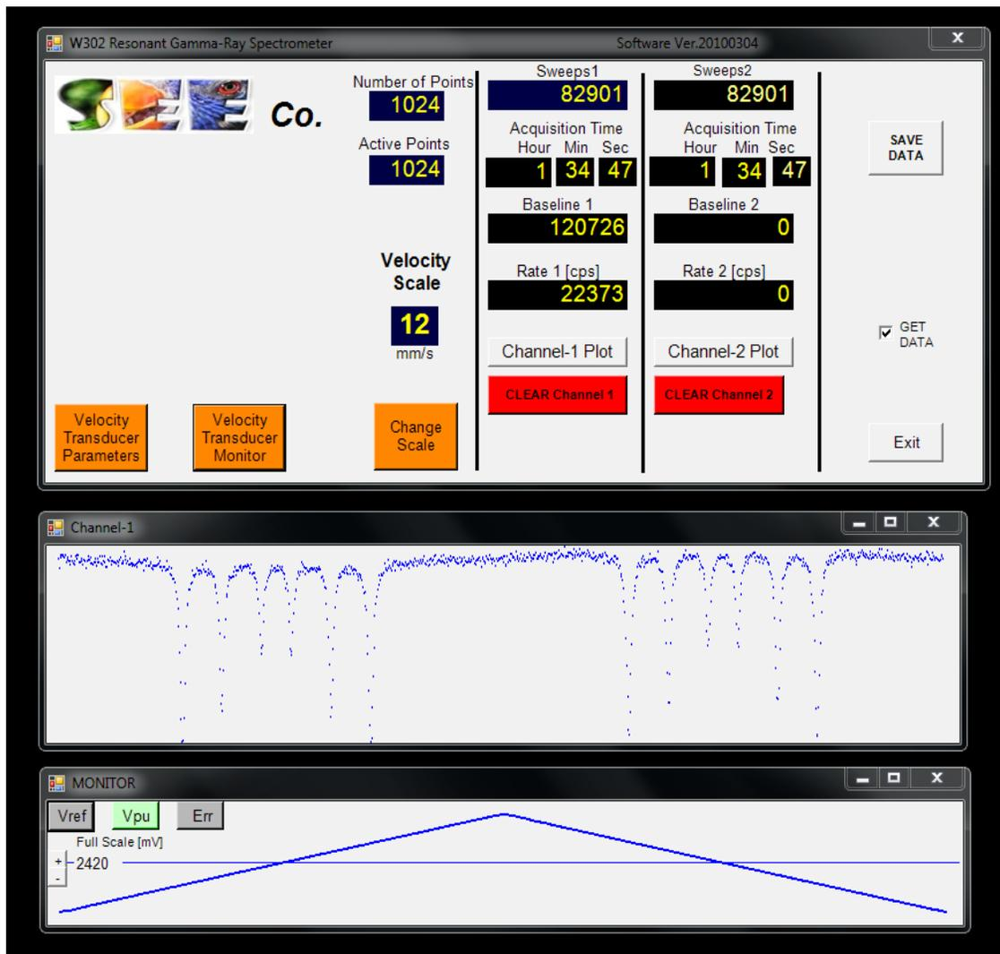
Figure 7. Screen with Main Window, Channel 1 Data Plot Window and Monitor Window.
