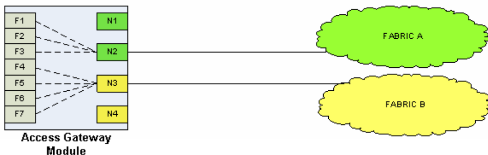
Figure 77 Part II: N_Port failover in an Access Gateway module attached to two fabrics (after N1 and N4 go offline)
