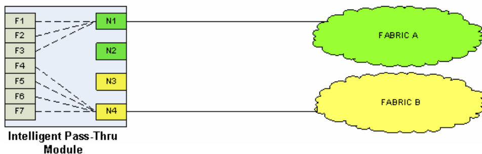
Figure 80 Part III: N_Port failover in an Intelligent Pass-Thru module attached to fabrics A and B (after N2 and N3 go offline and the primary and backup port settings have changed)
