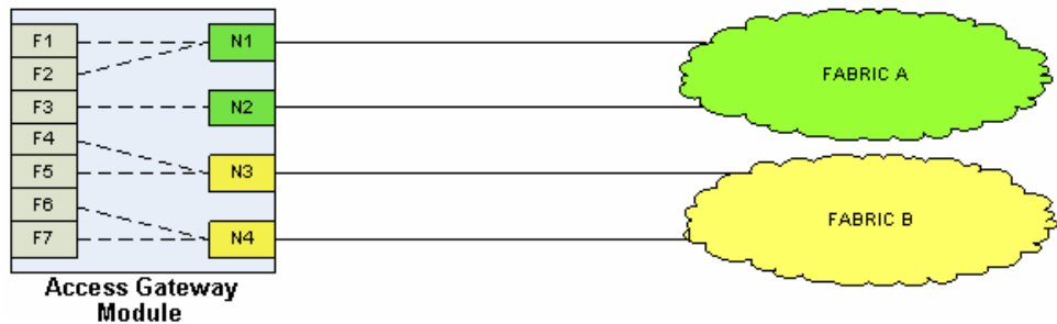
Figure 76 Part I: Access Gateway module attached to two fabrics
