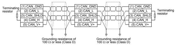
For electromagnetic compatibility (EMC), it is recommended to ground the cable shield at both ends.
