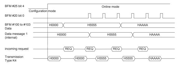
2) Transmission Type K4 (trigger via PLC/user flag)
