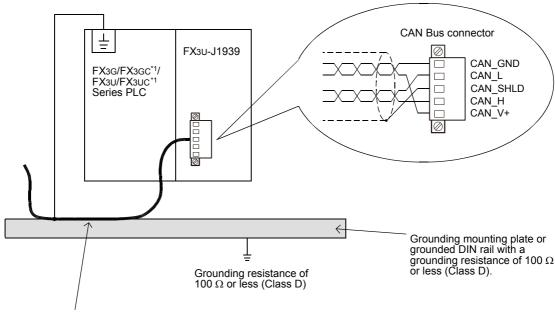
Strip a part of the coating of the shielded twisted pair cable as shown in subsection 4.2.3. Ground the PLCs grounding terminal there.
