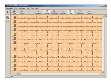
You can scale the ECG curves with zoom tool. The size of both full leads and median complexes changes simultaneously and as a result median complexes may not fit into the corresponding window. Double-click on the splitter bar between the **ECG Display Area** parts will change the width of median complexes area so as to make the whole length of complexes visible. At the same time, the width of median complexes part cannot exceed one third of **ECG Display Area** total width.
