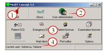
This is a starting window of seca CardioConcept programme. It is used for logging into seca CardioConcept database and launching various seca CardioConcept applications and utilities.
