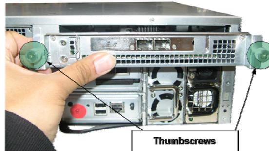
Figure 5.5: Removing/Inserting a 3U16 Auxiliary Module
