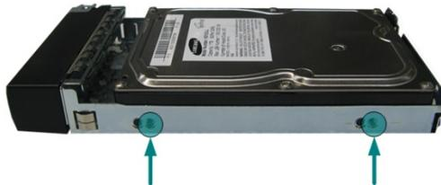
Figure 2.2: 3U16 SBB Drive Screw Locations (same applies to the other side)
