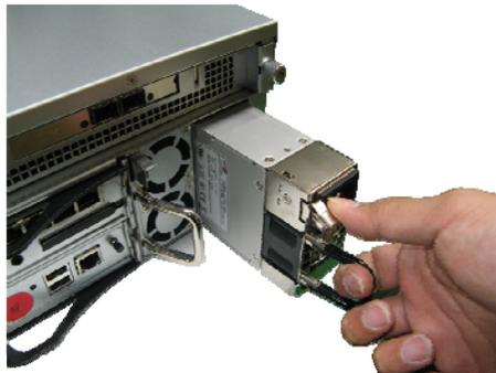
*Figure 2.5: A 3U16 PSU Module removed*
