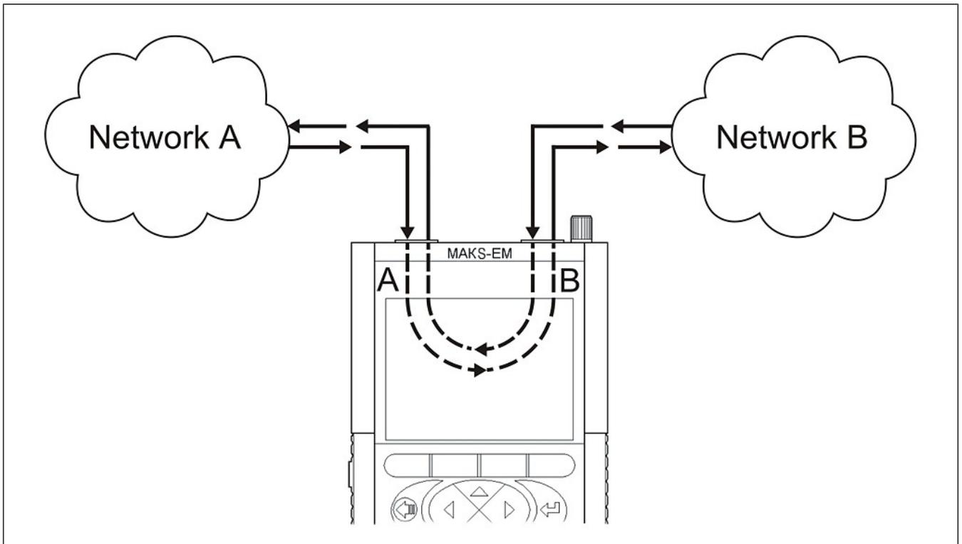
Figure 10.14 “Through” mode connection diagram
