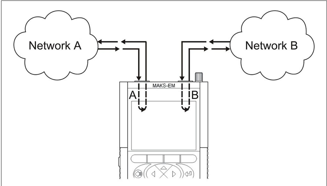
Figure 10.13 Loopback Mode Connection Diagram
