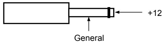
Figure 4.2 Soldered connections of power unit jack plug
