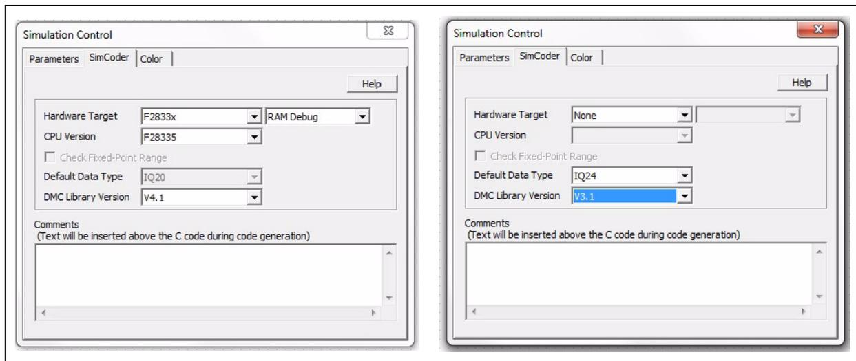
Go to the subcircuit's attributes dialog. Click on the **Generate Code** button and select **Generate Code for Hardware Target**.
