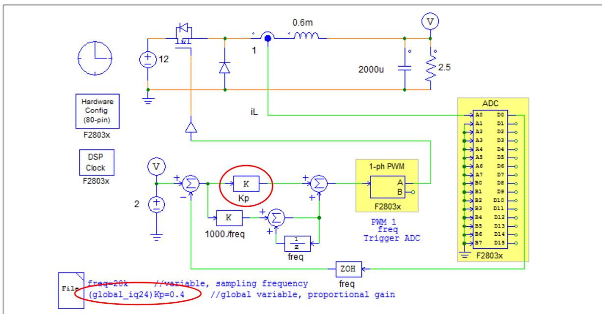
The generated code for F28335 is shown below. Note that in the code, the parameter  $K_p$  is defined as 0.4 at the beginning, and the parameter name  $K_p$  is used in the calculation.
