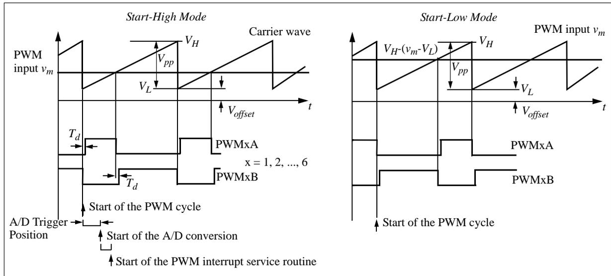
The figures above show how the dead time is defined, and the time sequence when the PWM generator triggers the A/D converter. If triggering the A/D converter is selected, from the start of the PWM cycle, after a certain delay defined by the A/D trigger position, the A/D conversion will start. After the A/D conversion is completed, the PWM interrupt service routine will start.
