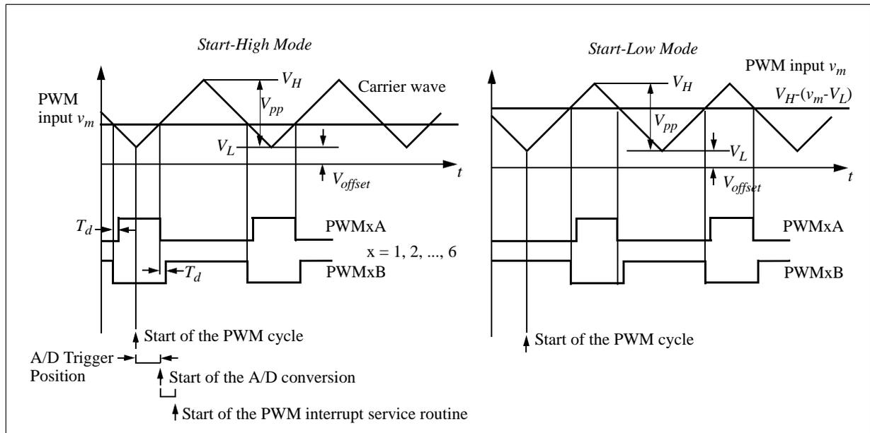
The input and output waveforms of a PWM generator with the sawtooth carrier wave are shown below:
