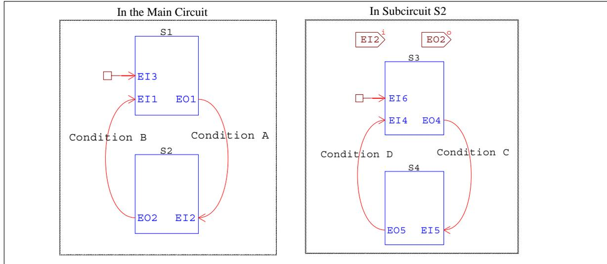
In the main circuit, there are two states: S1 and S2, both in the form of subcircuits. The schematic of each state is included in a subcircuit. State S1 has two input event ports: *EI1* and *EI3*, and one output event port *EO1*. State S2 has one input event port *EI2* and one output event port *EO2*. By default, State S1 is the default state at the beginning. This is defined by the connection of the default event element to the input event port *EI3*.
