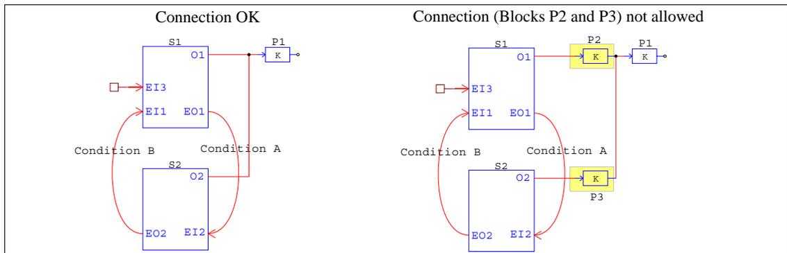
In the circuit on the left, both subcircuits S1 and S2 have one output signal port, O1 and O2. They are connected externally together to the input of the proportional block P1. The way the circuit works is that the input of the block P1 will come from either Port O1 or O2, depending on which state is active. This connection is allowed.
