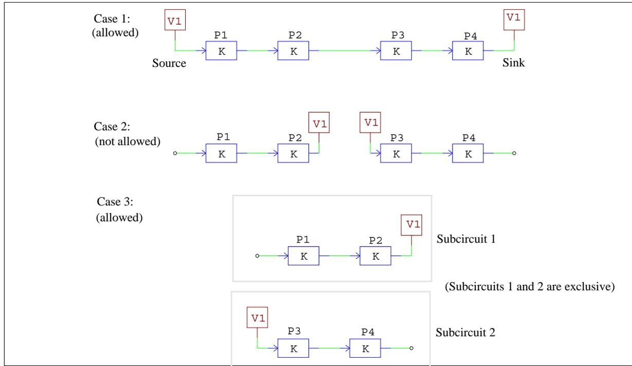
In Case 1, a global variable V1 is first used as a source and it assigns the value to the input of the block P1. After a series of calculation, the output of the block P4 is assigned back to the same global variable V1. Since both global variables are in the same signal flow path, it is allowed.
