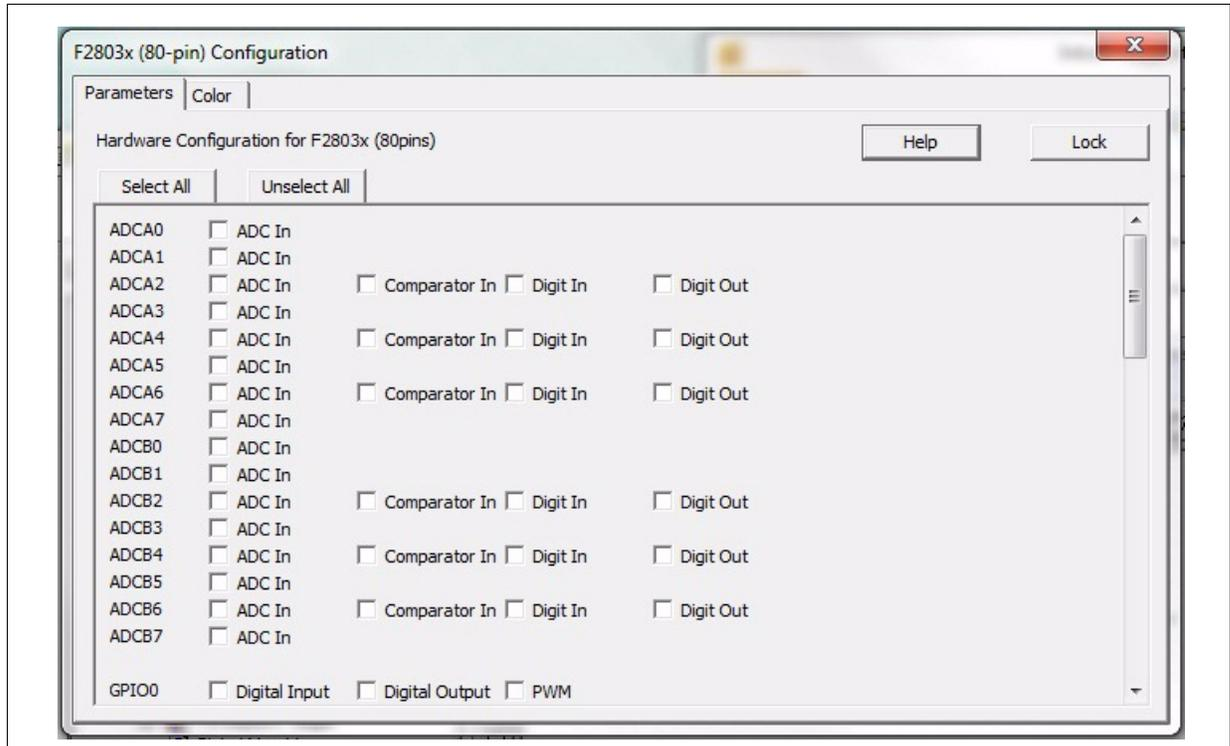
The Hardware Configuration block is for user to specify the I/O ports of the F2803x hardware. Every port to be used must be assigned correctly. The ports not in use can be left unchecked.
