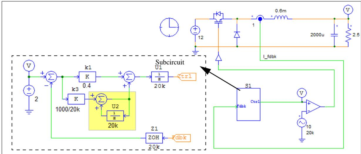
To create the subcircuit, select the circuit in the dotted box. Right click the mouse to display the pull-down menu. From the menu, select **Create Subcircuit**, and define the subcircuit file name.
