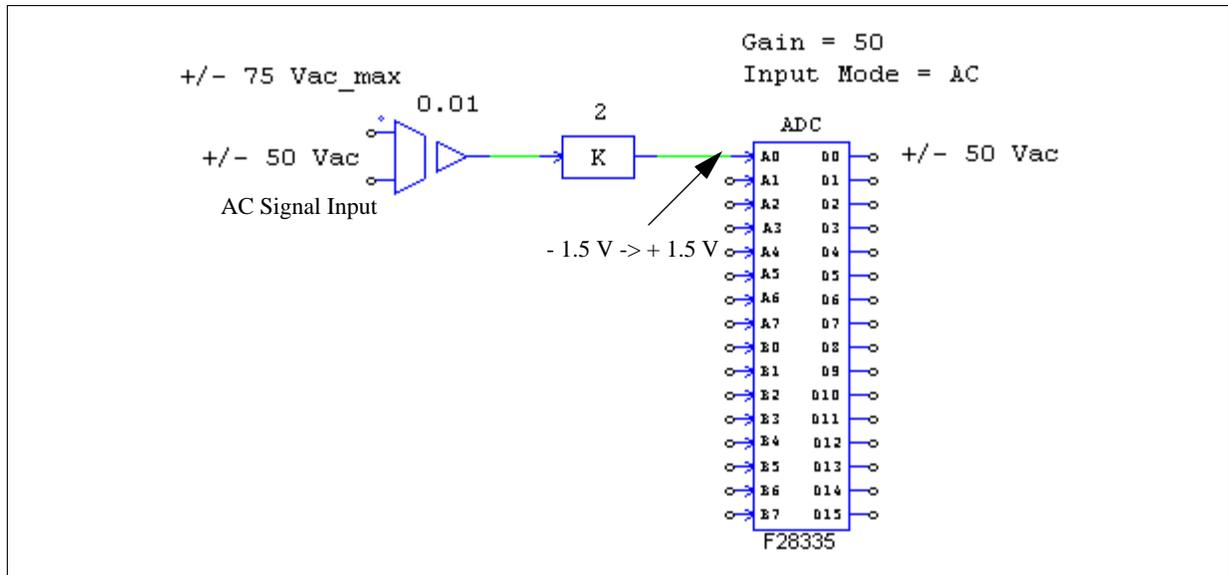
Notice that in this circuit, the ac signal is sent to the A/D converter directly. This is because that, when the A/D input mode is set to ac, the input range is from -1.5V and +1.5V, and the function of the conditioning circuit that performs the dc offset is already included in the A/D converter block. In the actual hardware circuit, the ac signal will need to be scaled and offset so that the range is within 0V to +3V required by the DSP A/D converter.
