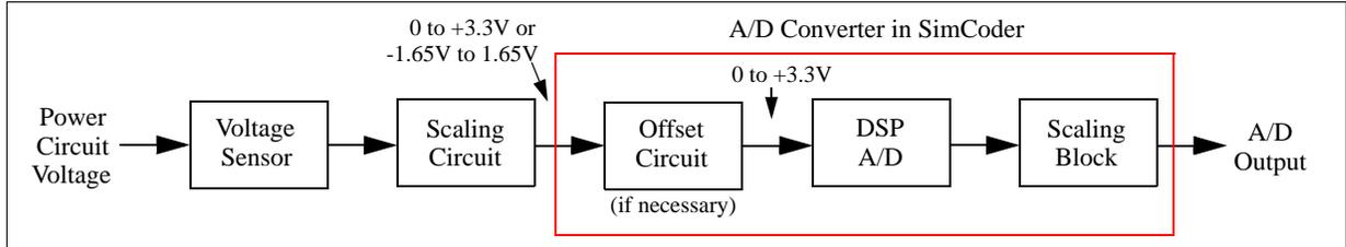
As shown above, the A/D converter element in SimCoder is not exactly the same as the physical A/D converter on the DSP. Rather, it combines the functions of an offset circuit, the DSP A/D converter, and a scaling block. This is designed for the convenience of AC system applications. It will be further explained in Section 6.5.3.
