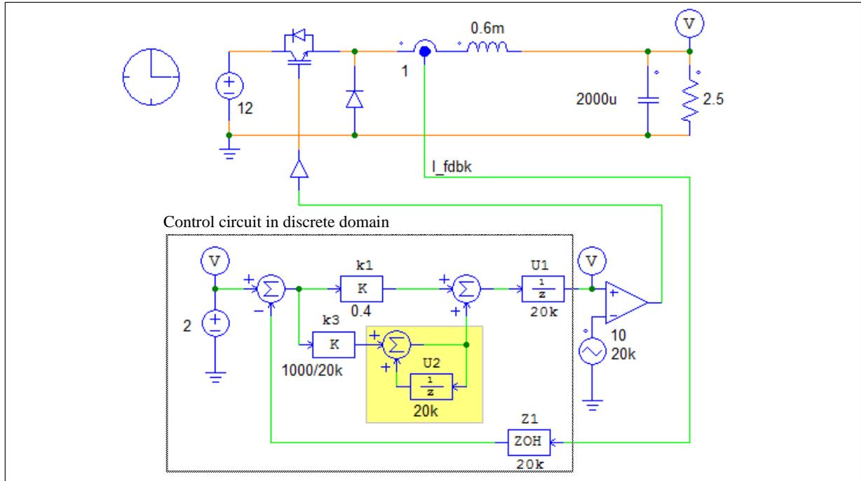
Note that, due to the factor  $T_s$  in the equation, the gain of the proportional block  $k_2$  needs to be divided by the sampling frequency of 20kHz. The advantage of this circuit is that it is easier to start or stop the integration of the integrator.
