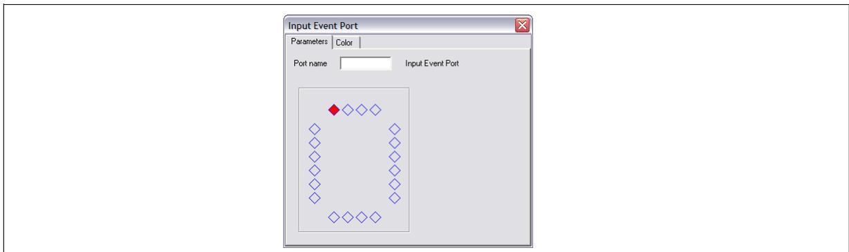
In the main circuit that calls this subcircuit, if there is an event connection wire connecting to this port, when the condition of the event connection is met, the system will transit to this subcircuit through this input event port.
