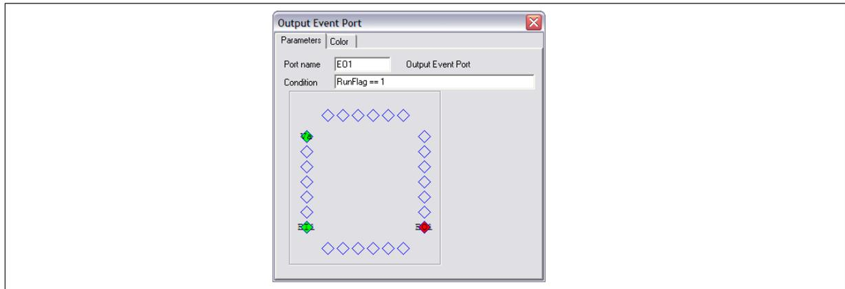
The condition "RunFlag == 1" is the condition that will trigger the output event to occur. The condition statement must be a valid C code expression. For example, the condition statement can be:
