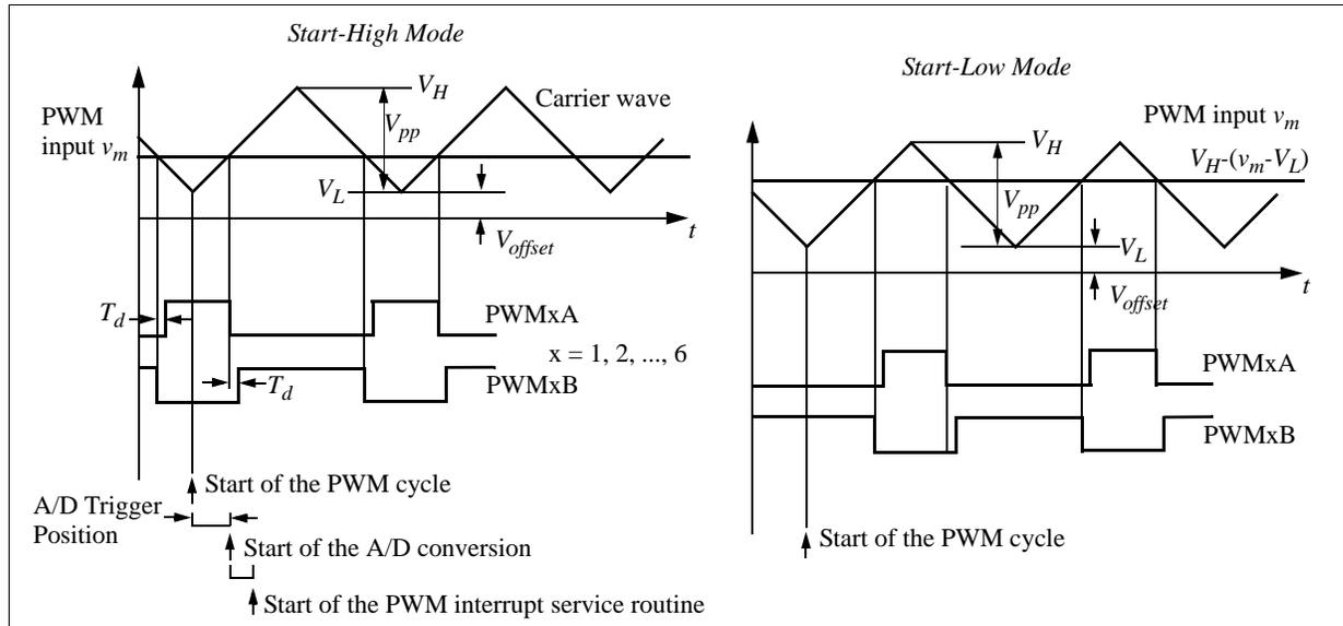
The input and output waveforms of a PWM generator with the sawtooth carrier wave are shown below:
