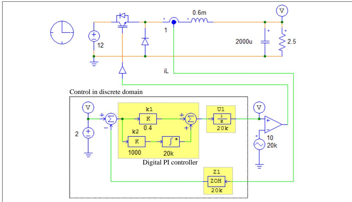
As compared to the control circuit in continuous domain, there are three changes in this circuit, as highlighted by the yellow boxes. First, the analog PI controller is replaced by the digital PI controller. The "Algorithm Flag" of the digital integrator is set to 1 (for Backward Euler method), and the sampling frequency is set to 20 kHz. The gains  $k_1$  and  $k_2$  are obtained from the conversion program as described above.
