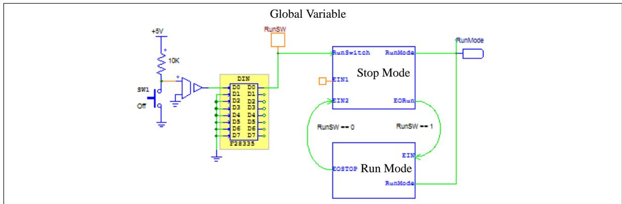
In this example, a global variable, *RunSW*, is connected to the output pin D0 of the digital input. This global variable is then used in the conditional statements between the transition of the two modes of operation.
