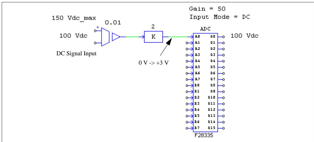
Please note that, in this example, if the gain of the proportional block is changed from 2 to 1, and the A/D gain is changed from 50 to 100, the simulation results will be the same. But the generated hardware code will not be correct. This is because the hardware code assumes that the maximum input value is scaled to +3V, but in this case it is only +1.5V. Therefore, one must set up the circuit such that, in the dc mode, the maximum input value is scaled to be +3V.
