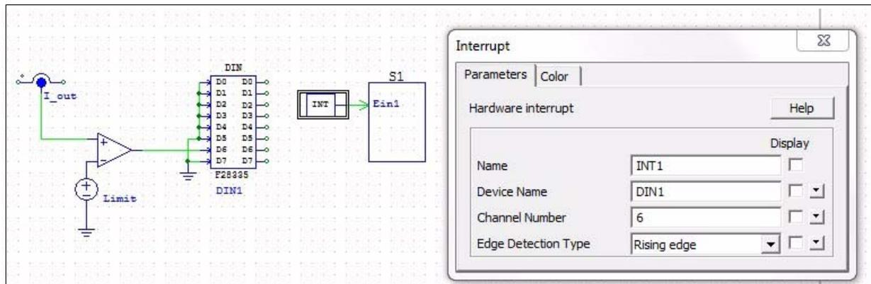
In this circuit, the current  $I_{out}$  is measured and compared with the reference value  $Limit$ . If the current  $I_{out}$  exceeds the  $Limit$ , the output of the comparator will change from 0 to 1. This will generate a rising edge to channel  $D6$  of the digital input block  $DIN1$ . The interrupt block parameters are set as shown in the graph:
