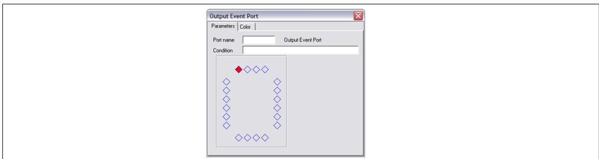
When the condition defined in the output event port is met, the system will transit out of this subcircuit into another subcircuit.
