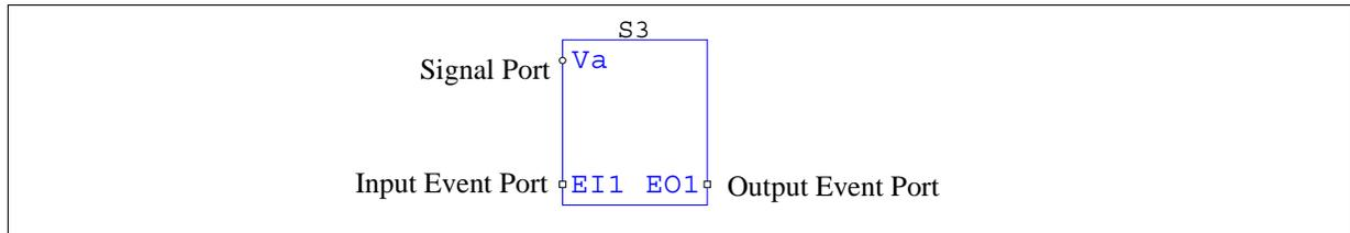
The image of an event port is a square, which is different from the image of a signal port which is a circle.
