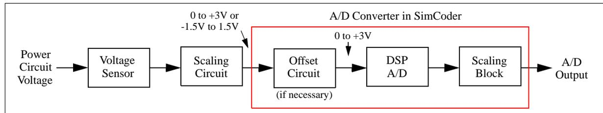
As shown above, the A/D converter element in SimCoder is not exactly the same as the physical A/D converter on the DSP. Rather, it combines the functions of an offset circuit, the DSP A/D converter, and a scaling block. This is designed for the convenience of AC system applications.
