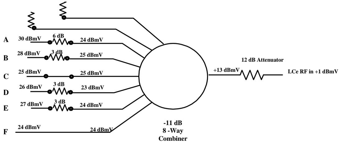
**Figure 3-2 Selecting Attenuation When Multiple Nodes Are Combined**
