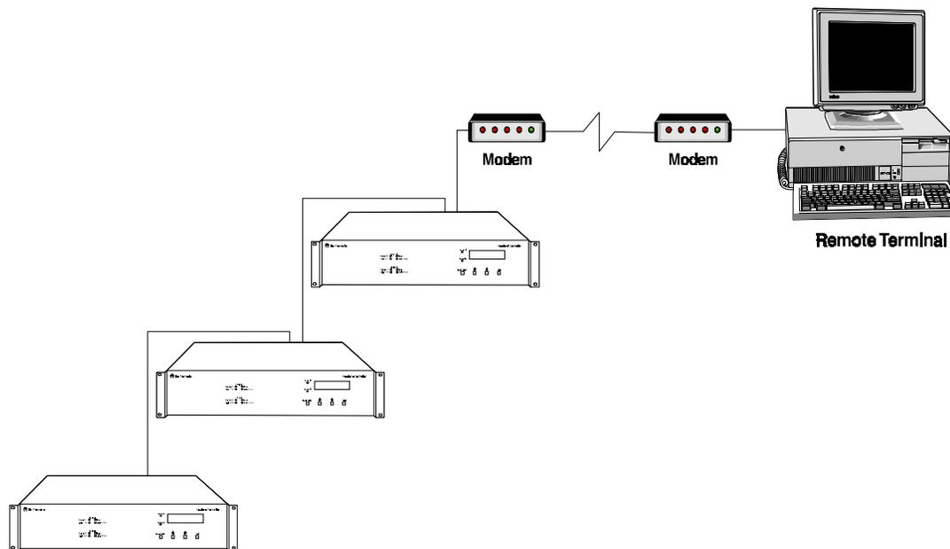
**Figure 4-3 LCe-4 Daisy Chain Cabling Example**
