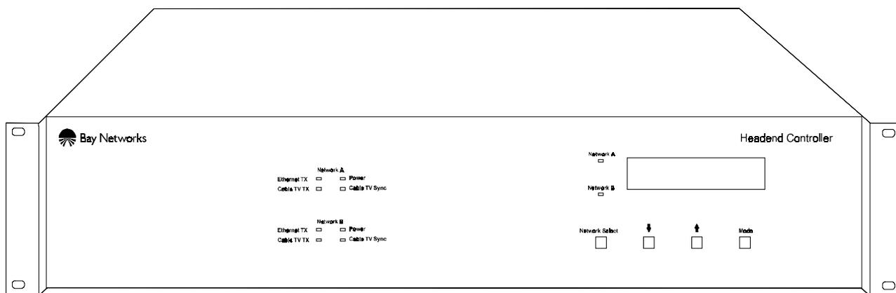
**Figure 1-1 LCE-4 Integrated Headend Controller**
