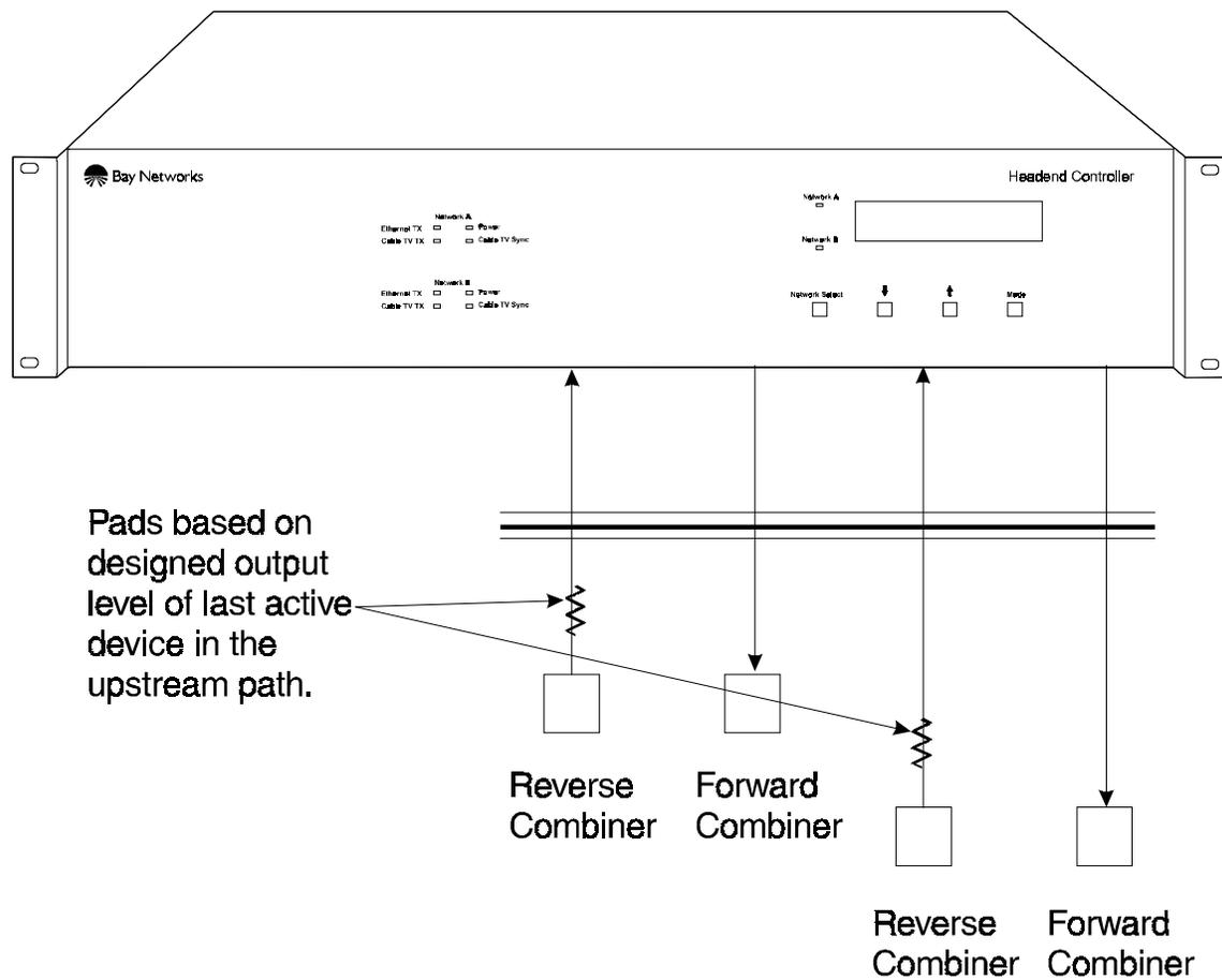
**Figure 3-1 Selecting the Reverse Channel Pad**
