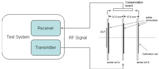
Bi-static Connection via ISO 10373-6 Standard Antenna
