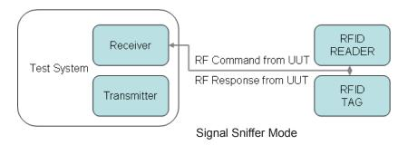
The test system will act as a third party sniffer, receiving the command and response signal between the reader and tag. The RF signal can be streaming to disk in real-time and playback later for post analysis. This configuration is suitable for RFID reader and tag system troubleshooting and application environment test.
