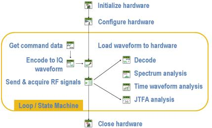
The typical data flow of the test toolkit is shown as the figure above, you may also start your 2<sup>nd</sup> development based on the source code of the Test Panel to build your own one.
