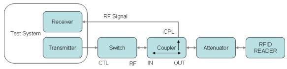
Mono-static Connection for Passive Tag Emulator
