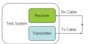
Receiver Calibration for Bi-static Connection
