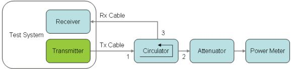
Transmitter Calibration for Mono-static Connection
