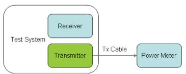
Transmitter Calibration for Bi-static Connection
