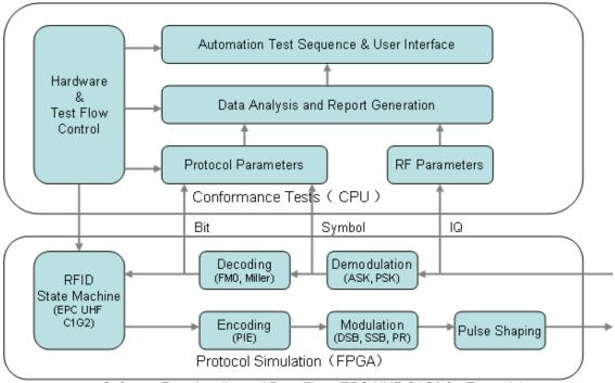
Software Functionality and Data Flow (EPC UHF C1G2 for Example)
