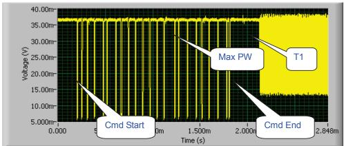
This method is suitable for most case except those special ones like "1 out 256 coding in ISO 15693". In this case the time interval between the Nth pulse and N+1th pulse inside a command frame might be longer than the specified T1, the parameter "Ignore Pulse" will help the system to determine what to do when T1 expired.
