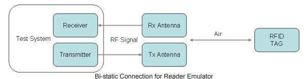
The bi-static connection via antenna and air interface is shown as above. Both the Tx and Rx antenna shall be wideband antenna which are capable to cover all the center frequencies under test. The recommended setup of the antenna and the EUT is, place the antenna side by side, face to the EUT.
