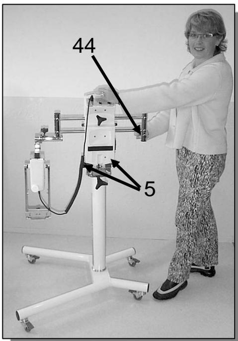
For easy transport, the unit features 4 wheels with brakes and the sliding motor mount bar (44) that also functions as a handle.
