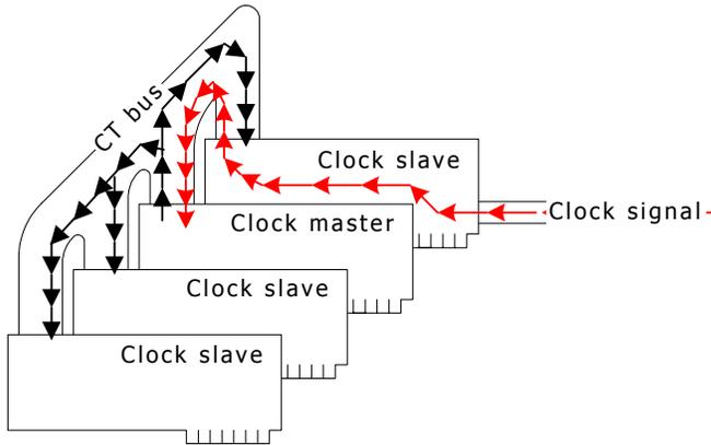
The channel over which the timing reference signal is carried to the clock master is called NETREF. The following illustration shows a system using a timing reference from NETREF:
