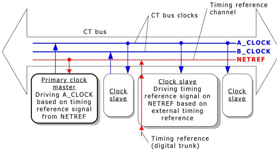
On the H.110 bus, a second timing reference signal can be carried on a fourth channel, called NETREF2. NETREF is referred to as NETREF1 in this case. The following illustration shows a system using a timing reference from NETREF2:
