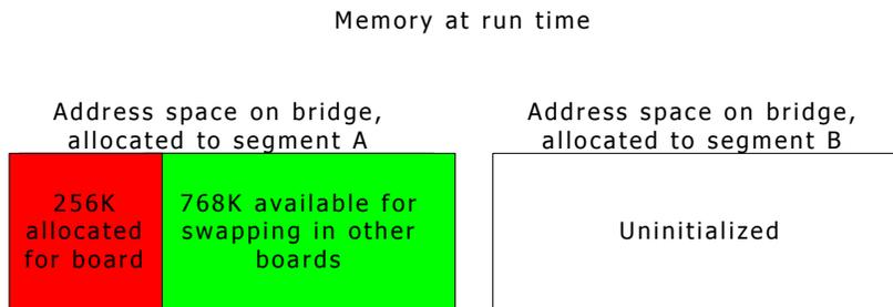
However, if an 8-slot segment has four slots occupied at boot time with the boards, no more boards can be hot-inserted into that segment because four boards occupy exactly one megabyte of address space. The following illustration shows a PCI bus with four 256K boards inserted:
