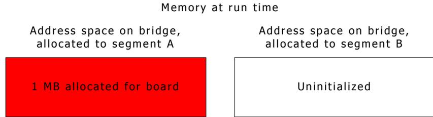
Some boards (such as the CG 6000C board) have an address space requirement of two 1 MB memory regions. Since this requirement exactly matches the 1 MB granularity, you cannot add more of these boards than were present at start-up without rebooting. The following illustration shows a PCI bus with a CG 6000C board inserted:
