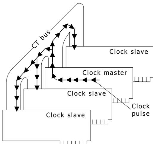
Two CT bus clocks can run simultaneously on the bus. They are called A\_CLOCK and B\_CLOCK. The clock master can drive either one. When you set up CT bus clocking, choose one of these clocks for your master and slaves. The other one is a redundant signal that can be used by a secondary clock master. Refer to *Secondary clock masters* on page 94 for more information.
