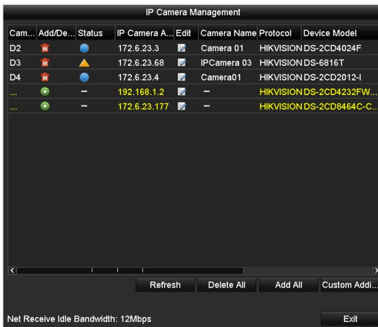
Figure 2. 14 Manual Adding IP Camera Interface
