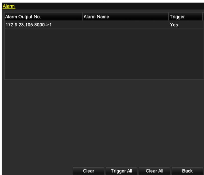
Figure 8. 18 Clear or Trigger Alarm Output Manually
