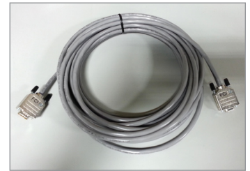
Amplifier to cabinet cable
