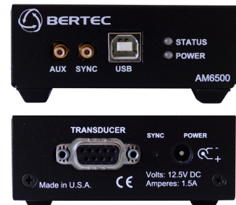
AM6500 Digital Signal Converter connections
