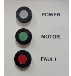
Electronic Control Unit Status Lights
