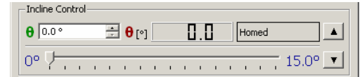
Incline Control and Drive Status section (Only available with a completely activated treadmill with the incline feature)
