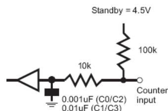
Maximum pulse rate to the counters is 20 kHz. Pulse rates must also be related to scan rate, to ensure counters do not overflow before being scanned by the PROLOGGER.
