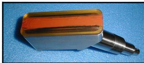
**Figure 1-9: Couplant on Transducer Face**
