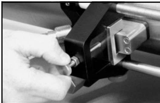
**Figure 1-10: Installing the First Transducer**
