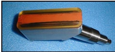
Figure 1-21: Couplant on Transducer Face
