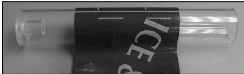
Figure 1-22: DMP-1 Damping Material Wrapped Around Pipe
