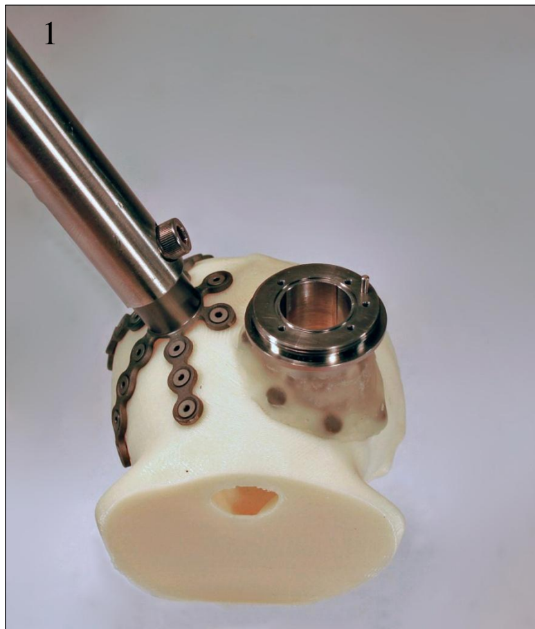
Step 1: Position skull model so that the chamber is vertically oriented.
