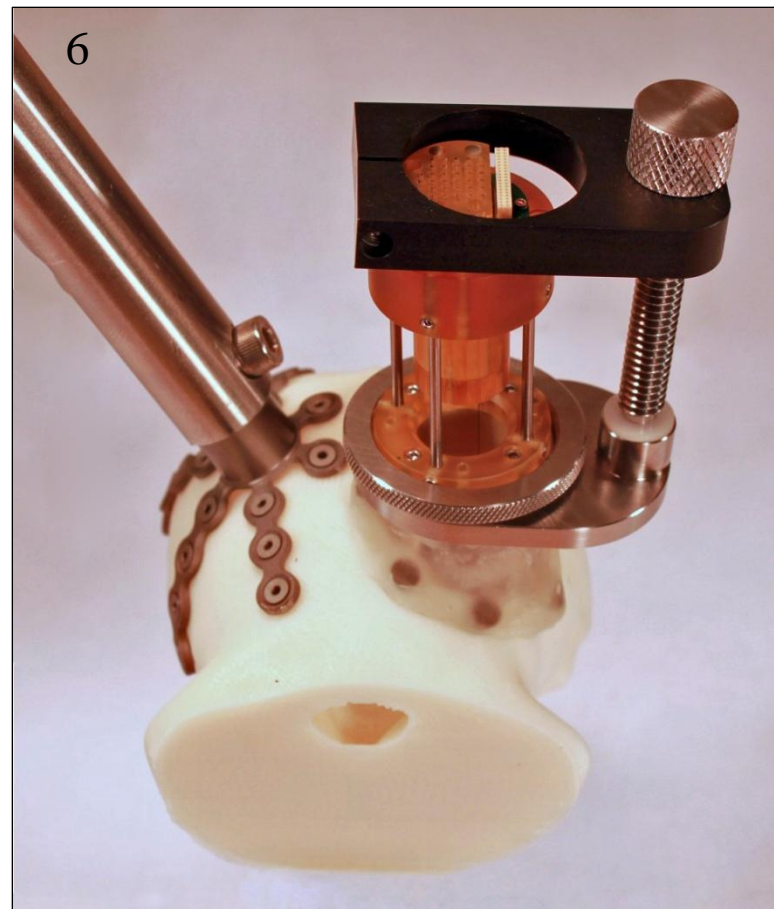
Step 6: Mount the coarse manipulator onto the chamber.
