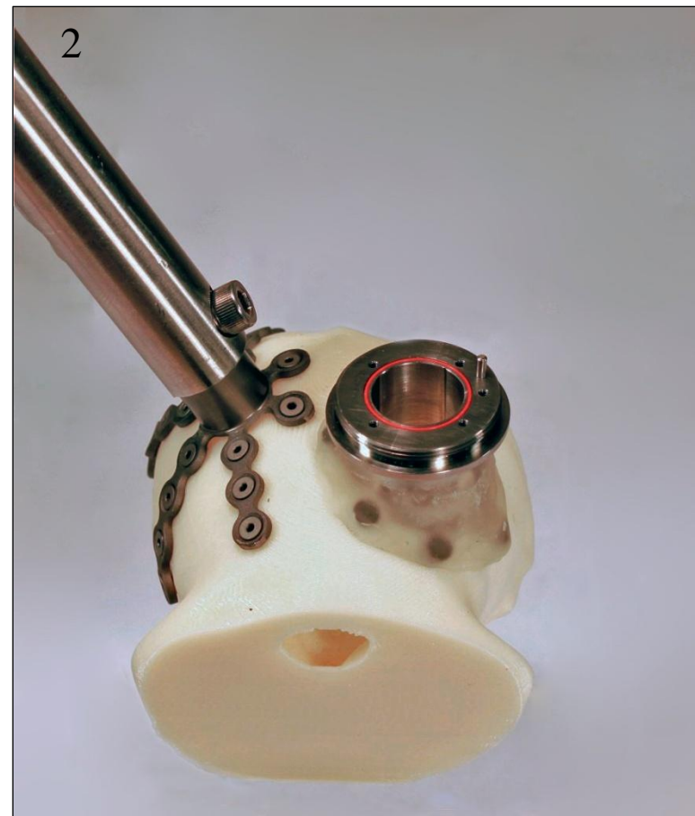
Step 2: Mount O-ring (red) within the groove on the top surface of the chamber.
