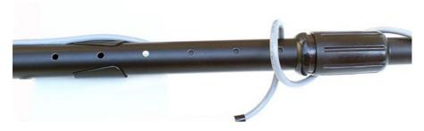
The Nexus Ultima is supplied ready assembled, with the telescopic stem retracted. To prepare the Nexus Ultima for use, simply extend the lower stem section and by using the locking pin underneath fix the two poles in working position to the desired length. Then tighten the locking collar to eliminate movement between the two parts of the stem.
