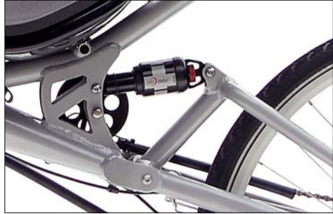
Air Shock DT-Swiss XM180. The damping is adjusted with the red wheel at the rear end.
