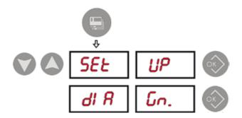
In the self-diagnostics sequence, all the LED's on the panel light up for a few seconds in order to check operation. When the LED's go out, the machine automatically moves on to the encoder reading phase. When the wheel is turned manually (forwards and backwards), the display shows its exact position. The value lies between 0 (zero) and 255.
