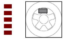
If "OPPOSITE POSITION" is enabled, the phase displays also indicate the weight application position at the bottom (6 o'clock) to facilitate cleaning the rim and the relative application of adhesive weights. The symbol used is:
