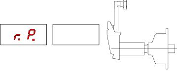
4. Bring the gauge in line with the adapter flange and press
