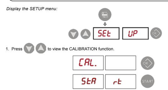
2. Add a standard weight of 60 g (2.00 oz) to the outer side, in any position. Failing a weight of 60g (2.00oz) press to change the calibration weight from 40 to 100g (1.40 to 3.50oz)
