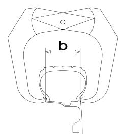
b) adhesive weights: make two successive measurements on two correction planes inside the rim.
