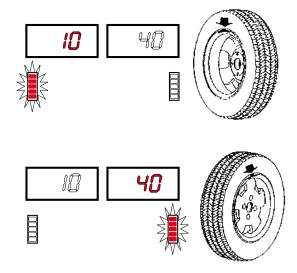
Move the wheel manually until all the LED's corresponding to the side light up. The display shows the measured unbalance. If the wheel clamp option is enabled (see **MENU**), the wheel is automatically clamped in
