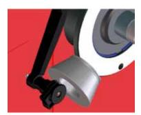
5. The number  $254 \pm 3^{\circ}$  should appear on the left display. The calibration is already correct.
