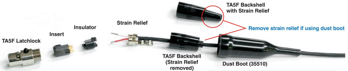
Note: If you use the dust boot, remove the rubber strain relief that is attached to the TA5F cap, or the boot will not fit over the assembly.
