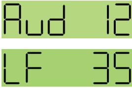
The Audio screen is used to adjust input gain from 0 to +44 dB, and the low frequency roll-off from 35 to 150 Hz. Repeatedly pressing the AUDIO button toggles back and forth between the two displays.
