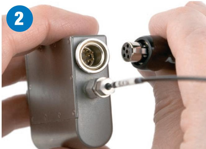
*Align the pins on the plug and jack and insert the connector.*
