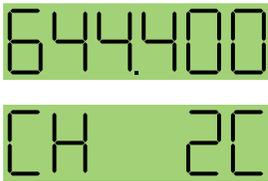
The Frequency Screen displays the operating frequency in MHz or as a two-digit hexadecimal number that corresponds to the equivalent Lectrosonics Frequency Switch Setting. Repeatedly pressing the
