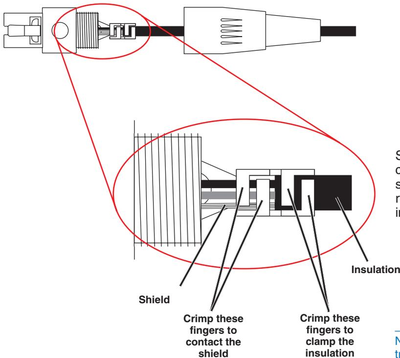
Strip and position the cable so that the clamp can be crimped to contact both the mic cable shield and the insulation. The shield contact reduces noise with some microphones and the insulation clamp increases ruggedness.
