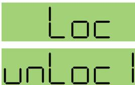
Simultaneously pressing and holding both the Up and Down arrow buttons during normal operation starts the Lock timer. The timer starts at three and counts down to zero. When the timer
