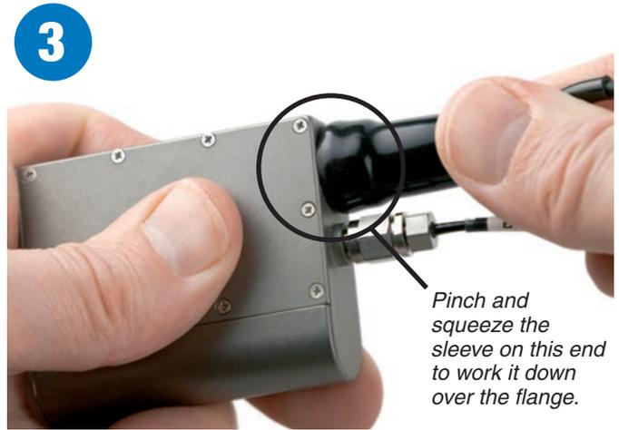
*Pinch and squeeze the sleeve on this end to work it down over the flange.*
