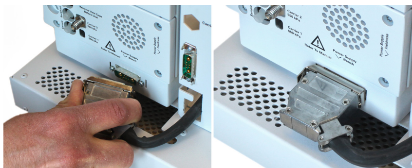
Figure 10 Squeeze the connector then push in
