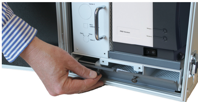
Figure 14 Unscrewing the nuts
