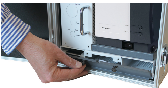
Figure 21 Unscrew the nuts
