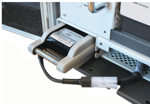
Figure 15 Install the battery
