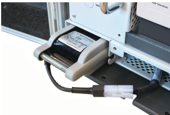
Figure 22 Slide out the battery
