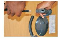
Step 2: Push the cable into the connector until you hear a "Click"
