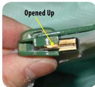
Fig. 26A. Zipper Slider Damaged from ripping the access panel open
