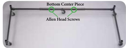
**Fig. 36. Allen Head Screw Location**
