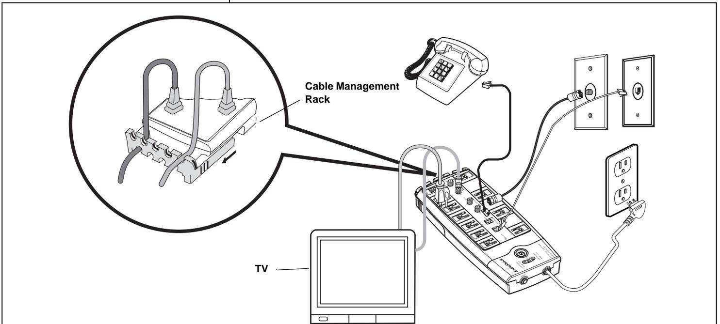
1. Connect one end of a modular telephone cord (not supplied) to the surge protector's **FAX/MODEM IN** jack, and the other end to a telephone wall jack.
