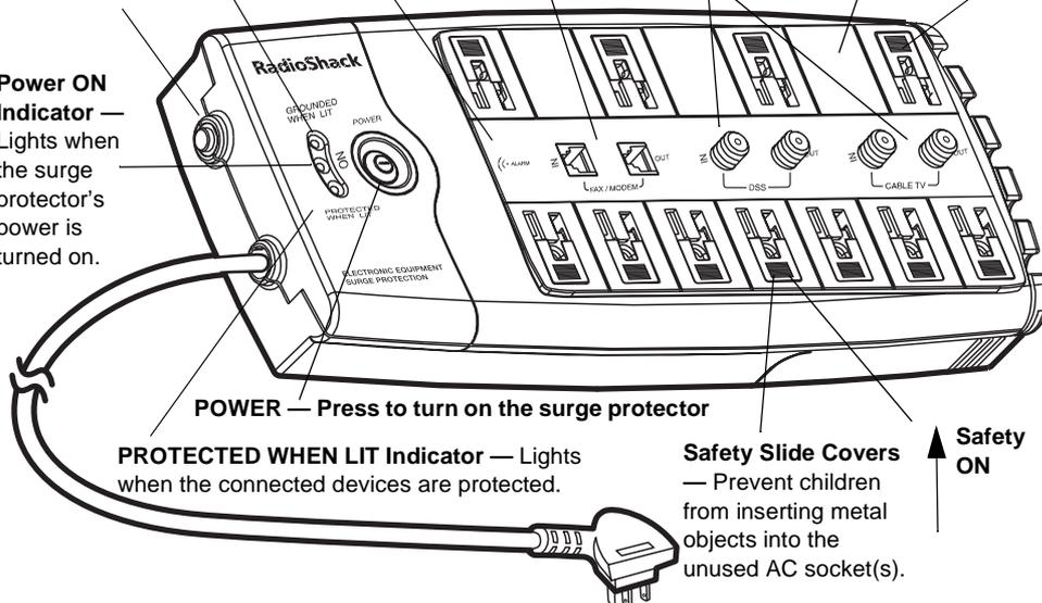
**PROTECTED WHEN LIT Indicator** — Lights when the connected devices are protected.
