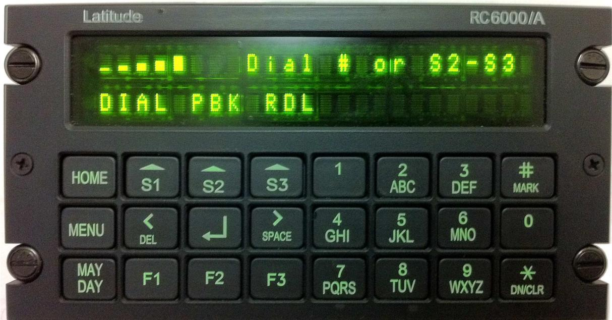
Figure 2 – Main Telephone Screen
