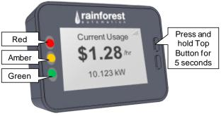
consumption is at the baseline rate or greater (up to 5x the baseline rate), the Amber light will be on. When consumption is more than 5x the baseline rate, the Red light will be on.
