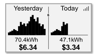
The graphs show hourly data, with a bar for each hour. The height of the bars is proportional to the number of kWh consumed for each hour. The graphs are auto-scaling, and meant to show relative, rather than absolute values. The small number
