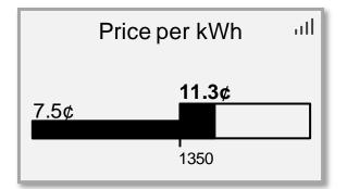
effect. When the threshold usage is reached, then the Step 2 price (shown on the right) comes into effect.
