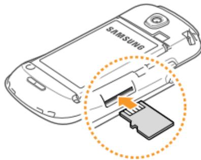
3. Push the memory card into the memory card slot until it locks into place.
