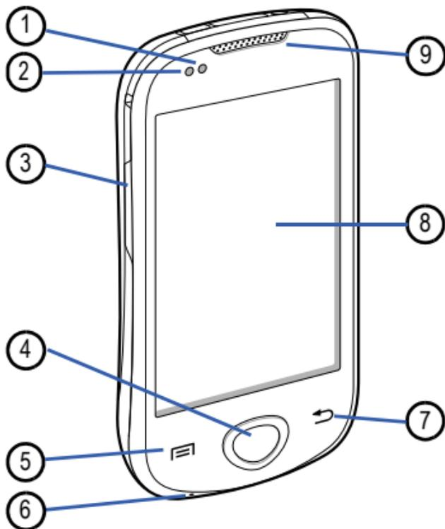
1. **Proximity Sensor:** Turns off the phone's touch screen display when a call is in progress.
