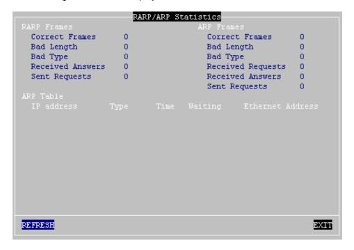
**Note**: the recognised '**IP Address/Ethernet Address**' associations are listed under these parameters. The 'Time' parameter is the number of seconds remaining before the Cache entry is deleted.
