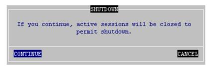
If the user confirms, all active connections (screen and auxiliary port) are closed. A few seconds later, the user is informed that the AX3000 may be turned off.
