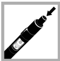
Figure 29 Dispense the electrolyte gel
