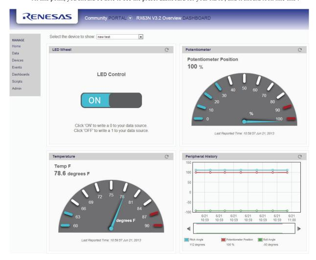
Go ahead and dial new input to the potentiometer, the temp sensor and the LED control button and witness the changes in the portal dashboard; response time may vary from several seconds to several tens of second based on the network performance.
