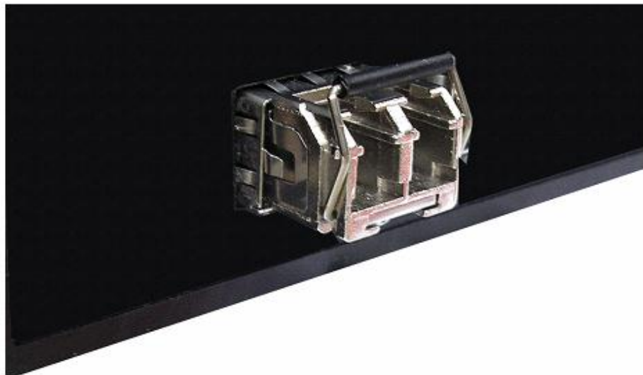
Figure - Insert transceiver into the SFP slot
