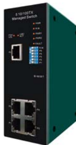
5 10/100TX with X-Ring Web Management Industrial switch
