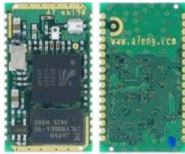
Figure 32. EmbeddedBlue eb100-SER OEM Bluetooth Serial Module
