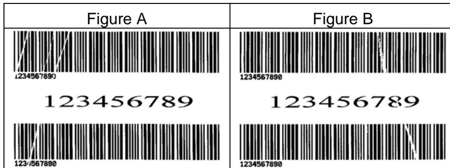
Once the printouts as above appear, the possible cause may be the unequal positions of Ribbon Bracket, which needs to be adjusted properly to make its heights equally the same at both sides. Steps to adjust are as below:
