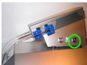
**Cable:** A 0.5 m cable connects the TIP2k to the Oxygraph-2k at the rear, with a 15 pin female SubD plug. When the TIP2k is connected to the Oxygraph-2k, and the mains of the Oxygraph-2k is switched on, the green light within the rear button on the side of the TIP2k lights up, indicating proper connection.
