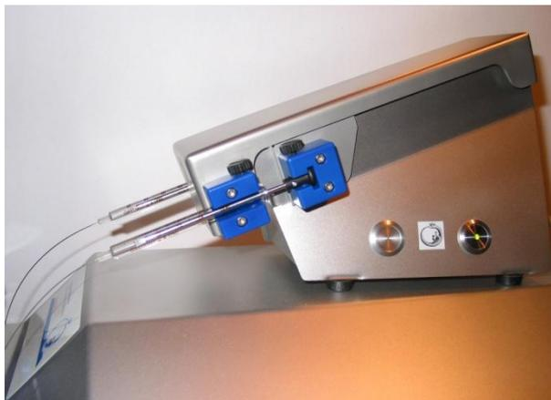
**Environment:** The TIP2k was tested at room temperature and must be protected from temperature fluctuations and condensation of water. The instrument must not be exposed to chemicals or vibrations, and the syringes should not be exposed to direct sunlight during operation.
