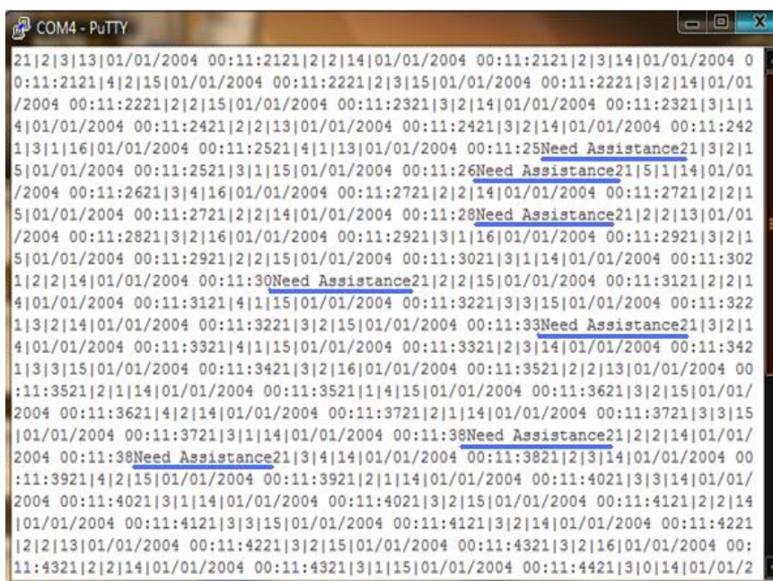
Figure 5-10: Data transmission in running session of PuTTY by using COM4
