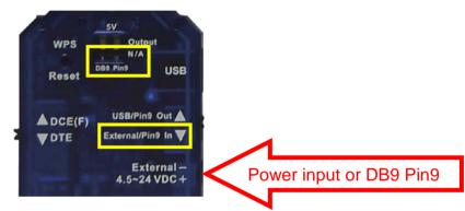
Remark: The power cable is used for the external power input which support larger range of voltage, 4.5~24VDC.
