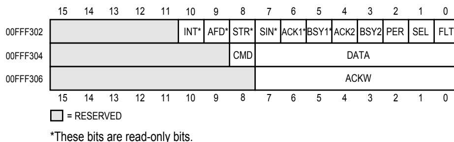
Figure 9-2. Parallel Port Interface Register
