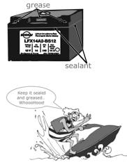
**A. WATER/CORROSION:** Avoid high pressure power washing around the battery case, or constant exposure to water. If the battery may be occasionally submerged, we highly suggest application of sealant to **fill the horizontal seam between top and bottom of the battery case**,
