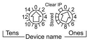
**NOTE:** Set the rotary switches before you apply power to the module and before you download the application.
