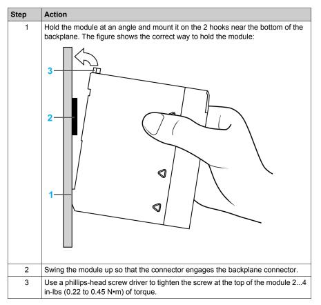
Use this procedure to install adapters and I/O modules in a rack:
