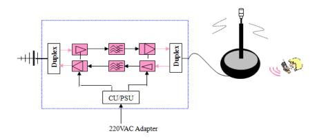
The signal from the base station is received via directly antenna, then forwarded through a duplex filter, is amplified in a low noise amplifier (LNA), enters the RF filter for wideband selective, and then amplified in the power amplifier.
