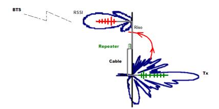
Isolation becomes particularly problematic when Omni-directional antennas are used for both the Donor and the Coverage antennas. Since these antennas transmit in a circle (or more accurately a sphere) it is very easy for these spheres to overlap and thus negate the repeater system.
